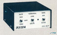
Interface to data terminal and two cassette recorders with a unit only 1/10 the size of SWTP's AC-30.
